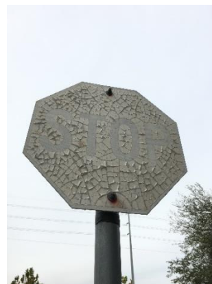
Heights Boulevard. Close-up of a weathered stop sign showing sun damage.
